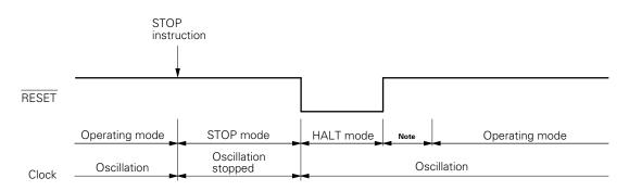
As soon as the RESET input makes a transition from high to low in the STOP mode, the system clock starts generating clock pulses.
